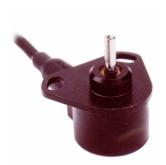
The output of a rotary potentiometer is a voltage which changes in direct proportion to the shaft angle. A constant voltage is required across the supply and ground wires of the sensor. No internal end stops are fitted, so continuous rotation is possible. The sensors are fully sealed against the ingress of fluids. Various lengths of electrically active track are available, up to a maximum of 348°.
